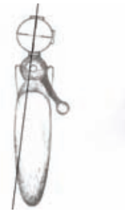
INCORRECT SCOPE MOUNTED ROTATED.
