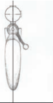
CORRECT THE IMAGINARY TAIL OF THE RETICLE CROSSES THROUGH THE CENTER OF THE BORE.
